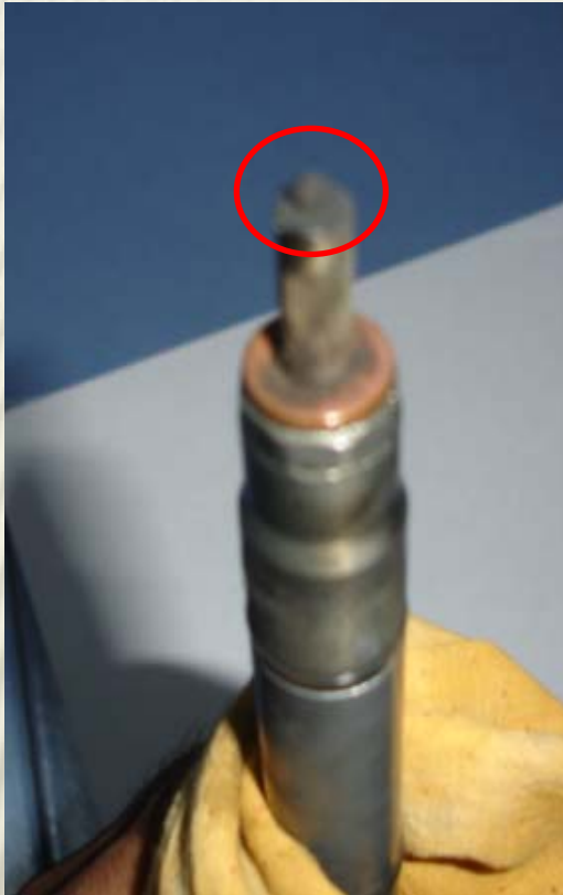
Heavily Scored Injector Pintle with Untreated Fuel
