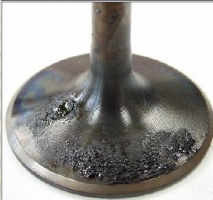
Heavily Scored Inlet Valve with Untreated Fuel
