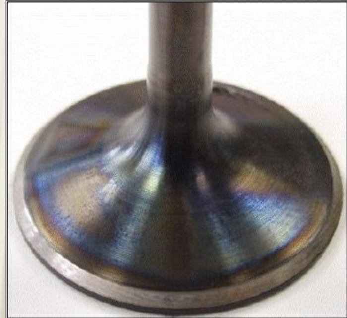
Clean Inlet Valve with additive treated Fuel
